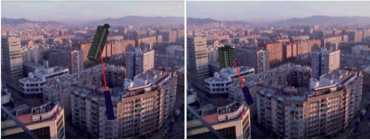
Figure 6 - Inserting a 3D model of a building into a video frame from Barcelona video. The user can move the model across the scene through a suitable interaction device (a symbolic representation of it has been super-imposed in the figure). The model is scaled according to its distance from the observer.
