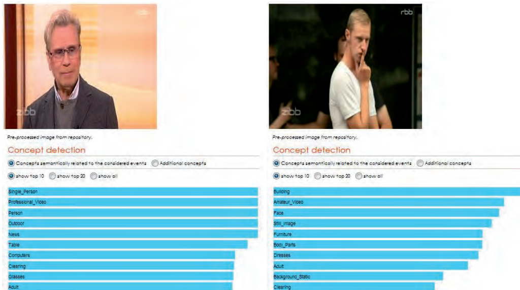
Figure 4: Top 10 TREC-Vid concepts detected for two example screenshots. Wrong concepts in the left one are “outdoor”, “table”, “computers”, and “clearing”, whereas the rest is correct. In the right one, only three concepts “face”, “body part” and “adult” are correct.
