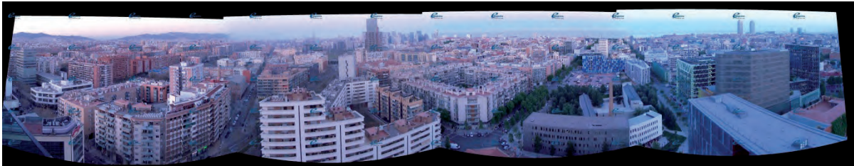
Figure 2 - Left eye frame of a panoramic view of the city of Barcelona. This image has been obtained by combining frames of four original, contiguous views. The geometrical distortion perceived in it comes after this stitching phase and it is due to the effort of matching corresponding points across two views.
