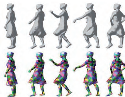
Figure 5: An example of mesh tracking (bottom) given independently estimated 3D models (top).
