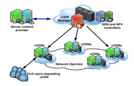
Fig. Virtual CDNs deployment model
