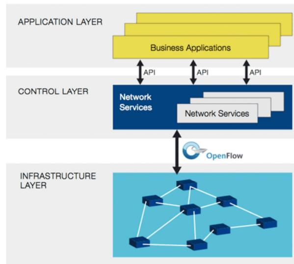
Fig: SDN Architecture (Source: ONF)
