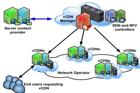
Fig. Virtual CDNs deployment model
