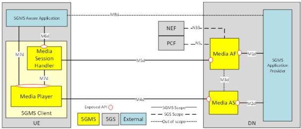
Figure 01 : High-level view of 5GMS downlink architecture
