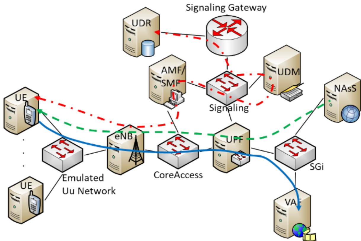
**Figure 1: Live Uplink Streaming Service (LUSS) on top of 5G network service**
